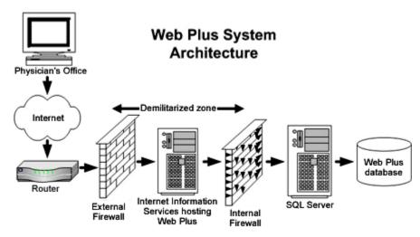
A router connects the demilitarized zone to the Internet. An SSL digital certificate is installed on the Web server for site authentication and encryption of data transferred between the clients and the Web server. The digital certificate can be created internally if a certificate server is available, or it can be purchased from a vendor. The organization needs to register a domain name if it has not done so already.
