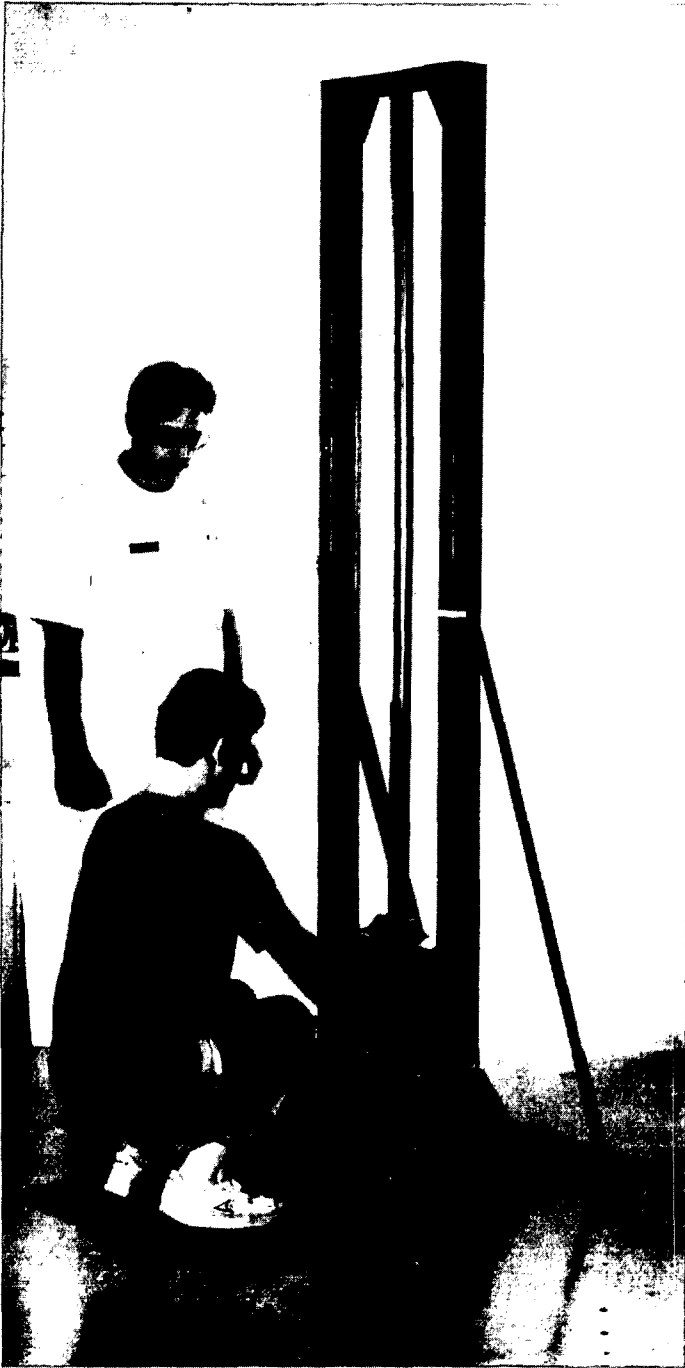
Figure 6. Incremental dynamic lift device used to determine maximal lift capacity.
