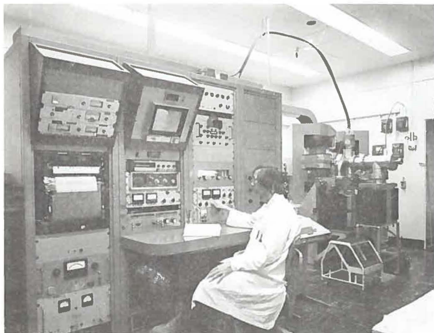
Fig. 4.10-15 Tandem solid-source thermal-ionization mass spectrometer in Room 216, CPP-602.
