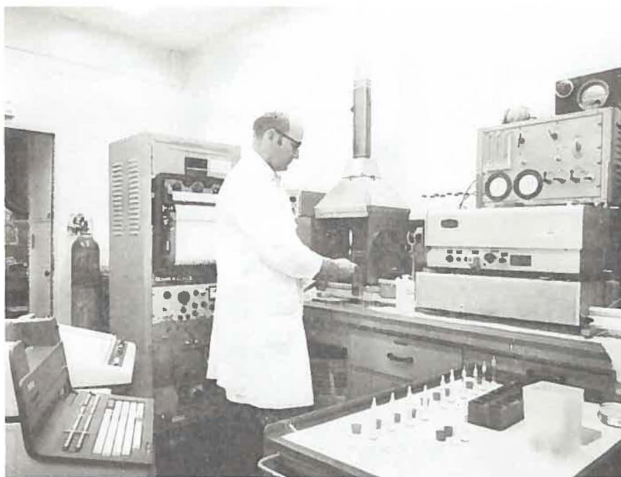
Fig. 4.10-21 Atomic absorption flame emission spectrometer in Room 227, CPP-602.
