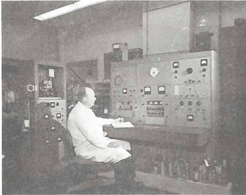
Fig. 4.10-16 Gas analysis mass spectrometer in Room 220, CPP-602.
