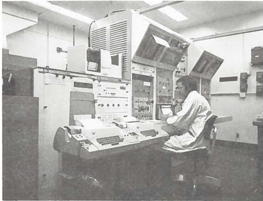
Fig. 4.10-11 Solid-source thermal-ionization mass spectrometers and on-line computer system in Room 212, CPP-602.
