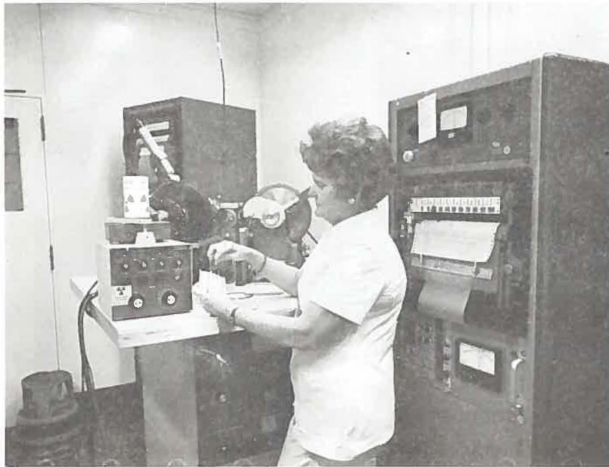
Fig. 4.10-22 X-ray generator with diffractometers and cameras in Room 315, CPP-602.
