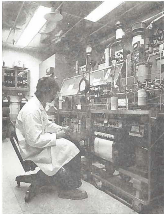
Fig. 4.10-2 Combustion trains for gas collection in Room 103C, CPP-602.
