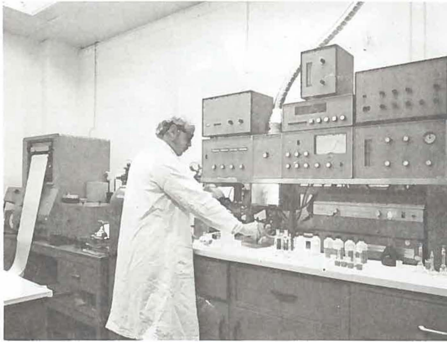
Fig. 4.10-12 Atomic absorption spectrometer and Cary recording spectrophotometer in Room 213; CPP-602.
