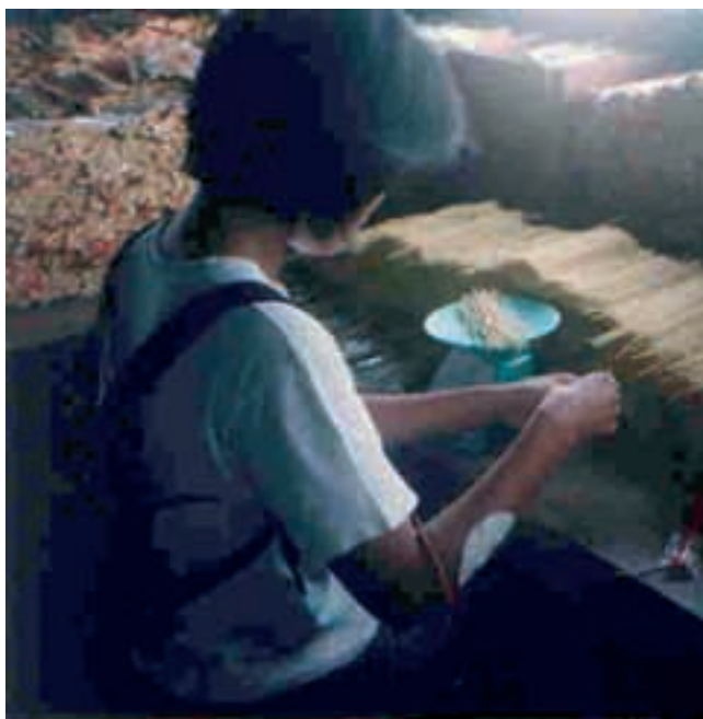
Before the improvement, the packing of noodles involved weighing the cut noodles with a scale.
