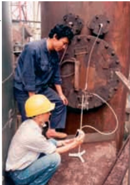
Taking air pollution samples at a workplace.
