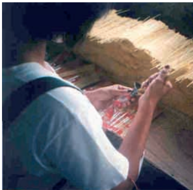
The use of a funnel in noodle packing, and elimination of the weighing shortened the operation time by over 75%.
