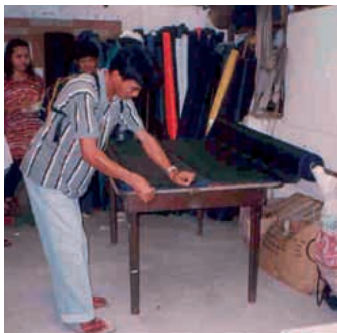
The metal frame at table height to hold the roll of material is a big help for the worker.
