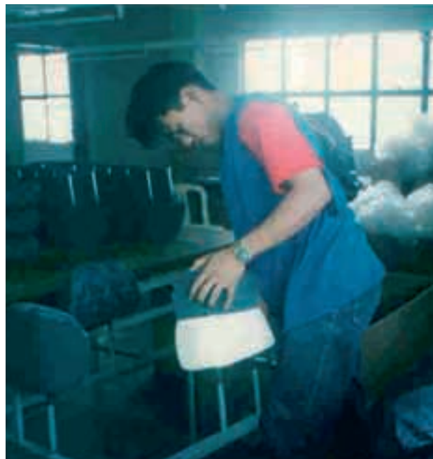
A fixture was constructed to speed up and facilitate the fixing of the cover of the headrest (picture on the right). The worker can now concentrate on fixing the cover. This was a worthwhile improvement.
