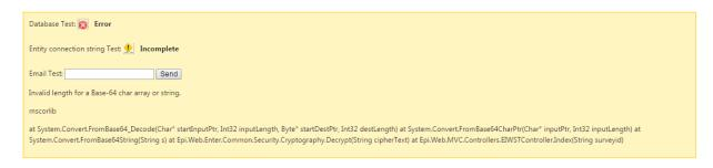
Figure 11: CRC eTool diagnostics view showing status when the application cannot communicate with the database server.
