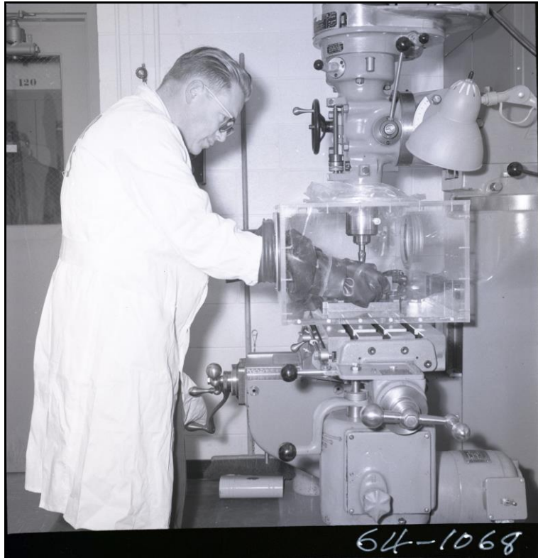
Figure 5-20: Scientist Machining Thorium, Alpha Lab, 1964
