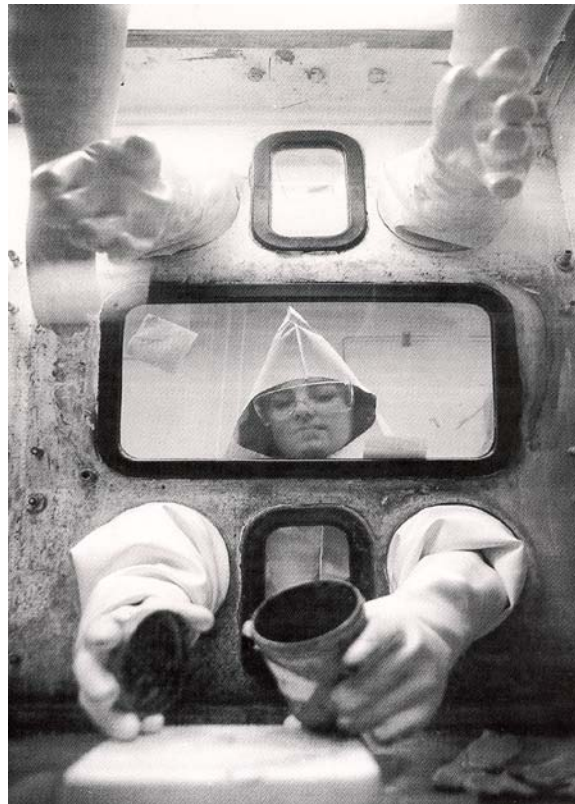
Figure 5 Other plutonium gloveboxes at Hanford. Note the viewing area in direct line with the lower torso in the center between the gloves. (2)
