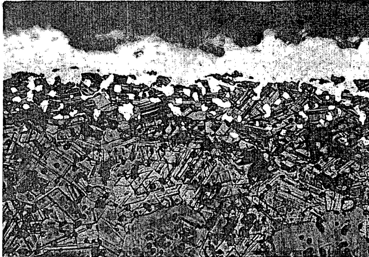
Fig 5.13 — UC Tested 1000 hr in Contact with Inconel-X — 500× — Nitric Acid-Acetic Acid-Water Etch
