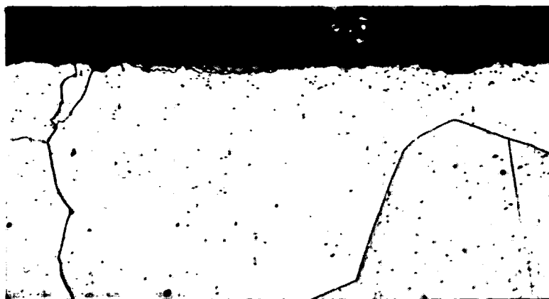
Fig. 5.12 — 2\frac{1}{4} Cr-1 Mo Steel Tested 4000 hr — 500× — Nital Etch
