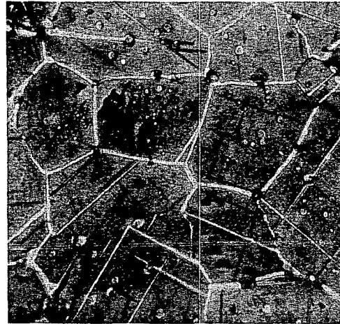
Fig. 5.6 — (U_{0.8}Pu_{0.2})C_{0.95} + 0.1 w/o Ni — Sintered in Helium and Vacuum Annealed at 1900°C, 1 hr. 600×. Etchant: Nitric Acid-Acetic Acid-Water.
