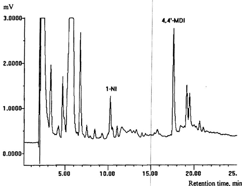
Figure 3. Example of liquid chromatogram for sample NCO13 containing 1.08 mg/kg 4,4'-MDI.
