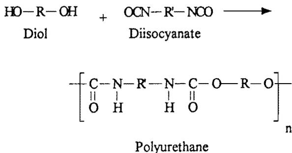
**Scheme 1.** Reaction of diol with diisocyanate to form a polyurethane of chain length  $n$ .
