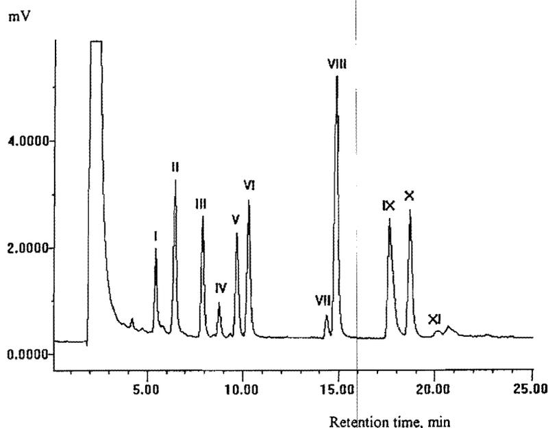
**Figure 2. Example liquid trace chromatogram for standard isocyanate derivatives: I, PI; II, CHI; III, 2,4-TDI; IV, 2,6-TDI; V, 1,5-NI; VI, 1-NI (internal standard); VII, 2,4'-MDI; VIII, IPDI; IX, 4,4'-MDI; X, HDI; XI, dimer.**
