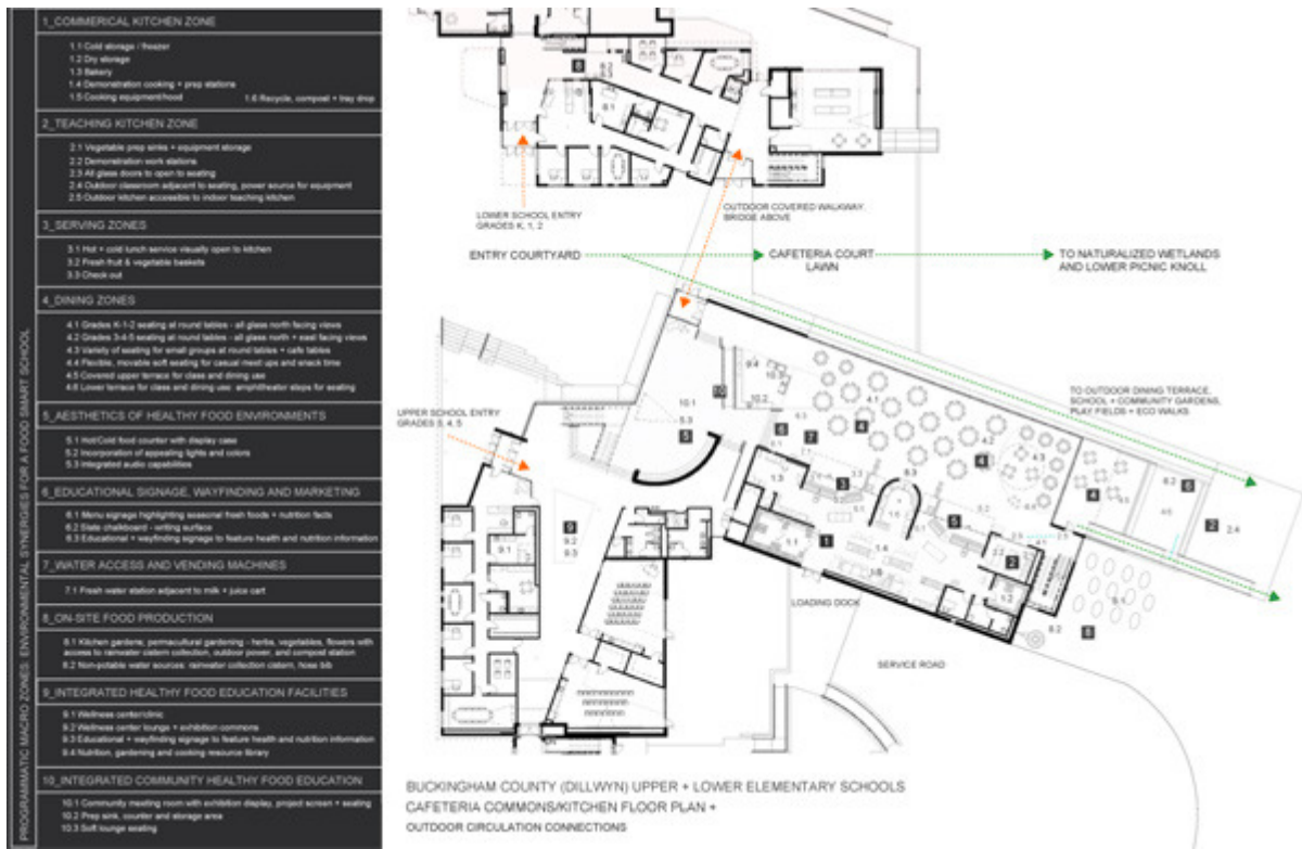
Figure 2. Floor plan for the cafeteria and kitchen for upper and lower elementary schools, Dillwyn, Virginia. [A larger copy of this figure with text description (PDF – 1.8 MB) is also available.]
